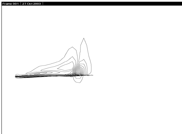
Fig. 11 Isovorticity contours ( \omega_x ) along the midchord line of forewing ( \omega_x : from -1 to 1 ) at kt = \pi (downward motion).
